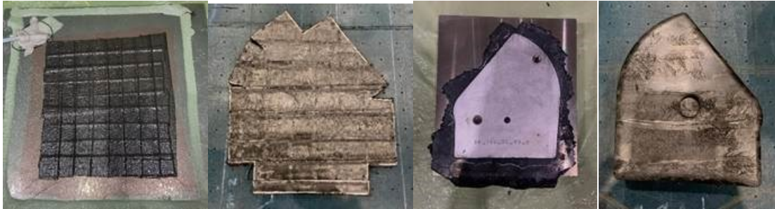
Figure 24: Manufacturing methodology for hot-press technology using reused material
