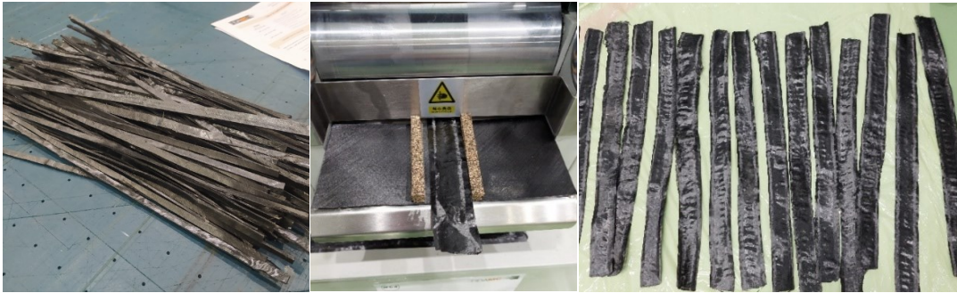
Figure 22: Calendaring method considering scrap as raw material, strip compaction and strip results
