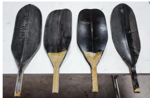
Figure 56. Thermoformed paddle with GF insert
