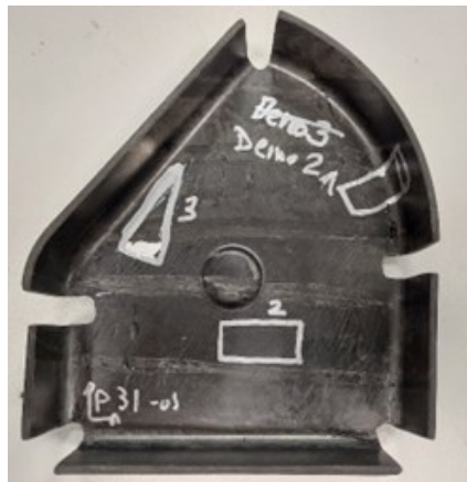
Figure 30: Demonstrator 2 manufactured using hot press process
