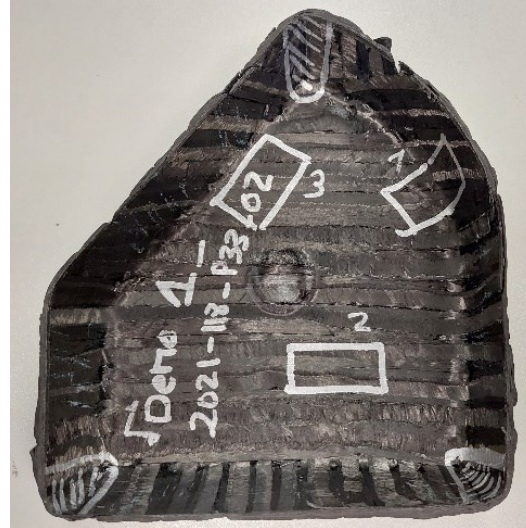
Figure 28: Demonstrator 1 manufactured by hand lay-up & vacuum bag
