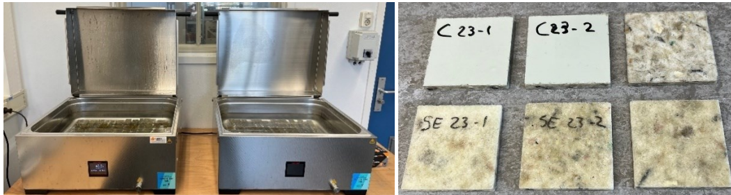
Figure 5 Test set up and sample for water absorption testing.
