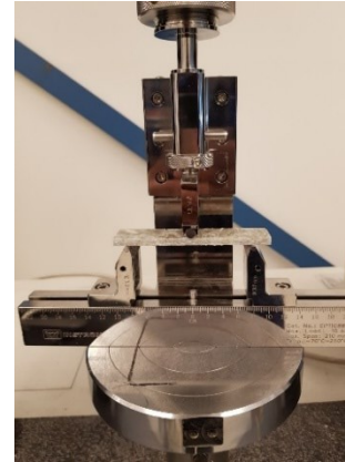
Figure 4. Set up for the three-point bending test
