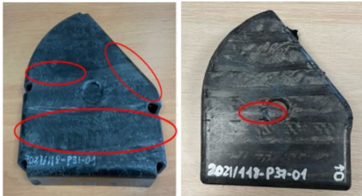
Figure 32: Comparison of dry spots and resin deficiency on the surface of Demonstrator 2 (3 plies, left) and Demonstrator 3 (2 plies,
