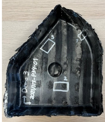
Figure 31: Demonstrator 3 manufactured using hot-press process and 2 plies
