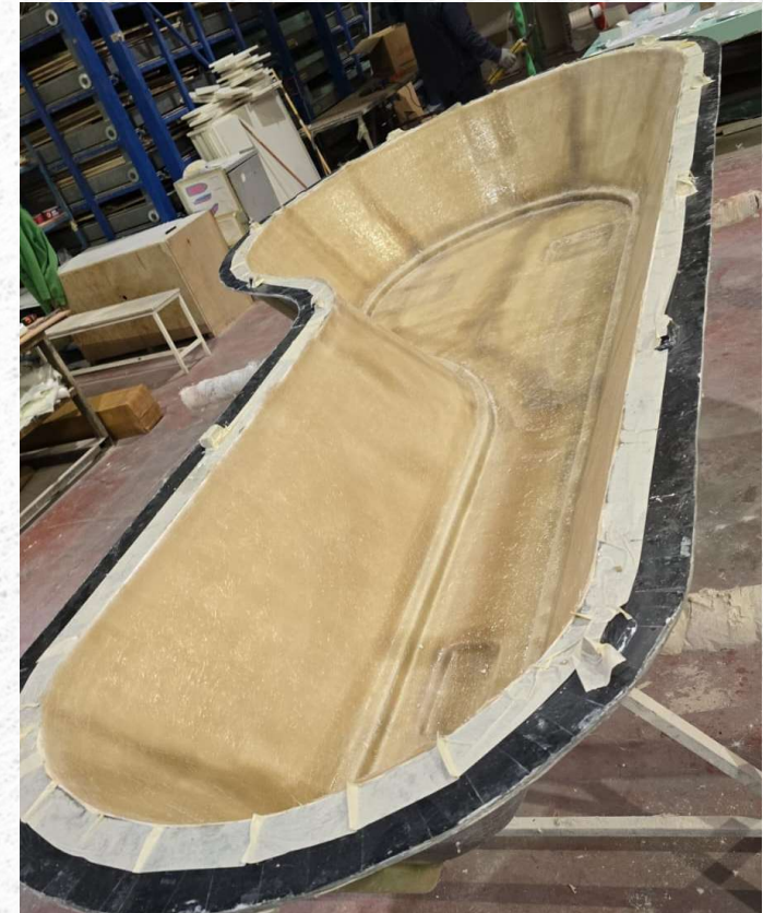
Image: Fiberglass layering
