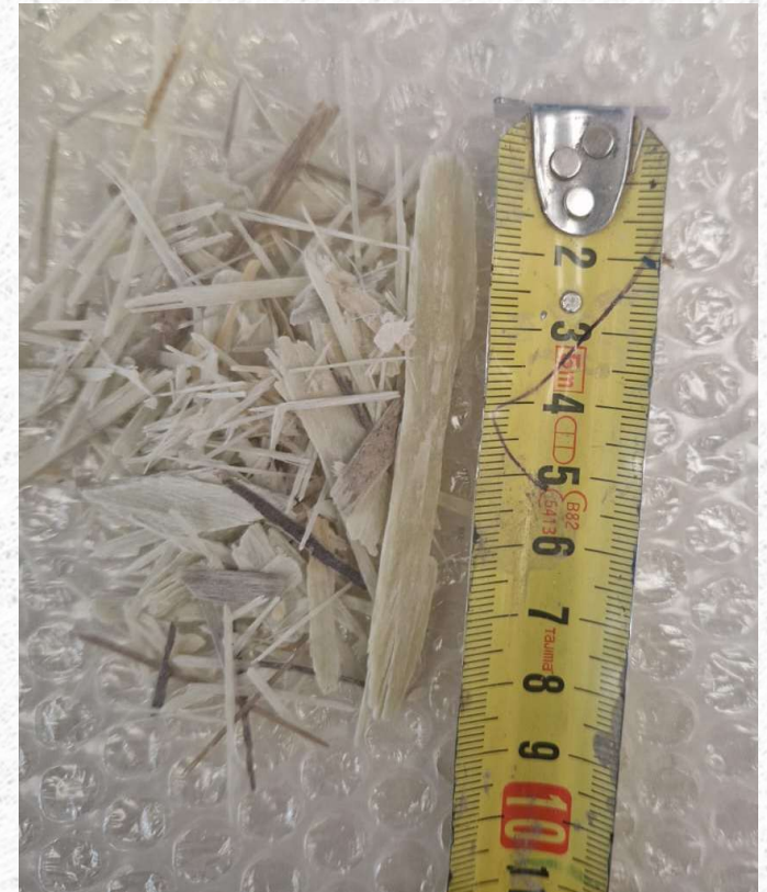
Image: Shredded GFRC granules
