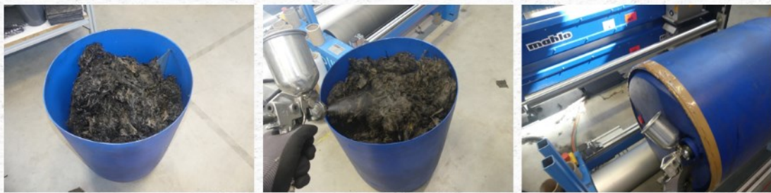
Figure 16: Resizing of solvolyzed carbon fibres from GAIKER
