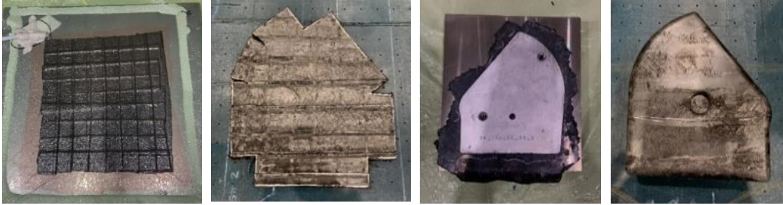
Figure 4: Manufacturing methodology for hot-press technology using reused material
