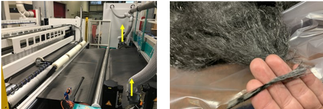
Figure 8: View on the extraction of cut edges on the NCF line at Chomarar by vacuum (Scheme: CHOMARAT)
